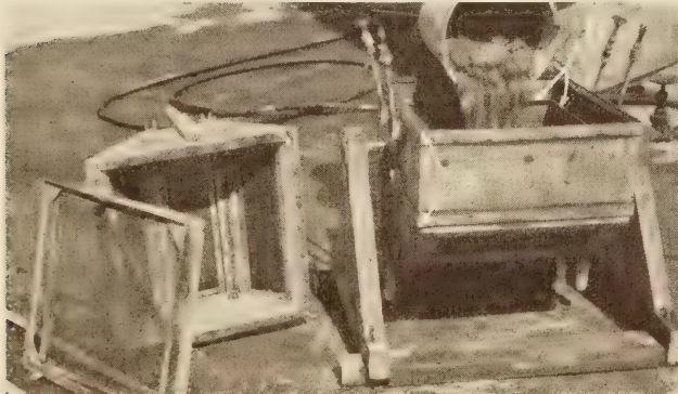
FIGURE 1.—THE SAMPLE OF FRESH CONCRETE TO BE ANALYZED IS PLACED ON THE NO. 4 SIEVE WHICH IS DIRECTLY BELOW THE PERFORATED PIPE AND ATTACHED TO BASE FRAME "A." ANOTHER SIEVE IS PLACED ON CLEATS "B" ABOVE THE PIPE
